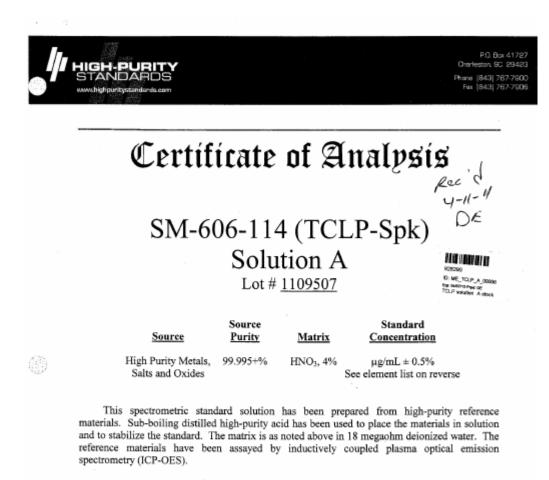
The standard has been prepared gravimetrically by weighing the reference material to 5 significant figures. Volumetric glassware has been calibrated gravimetrically to 5 significant figures. The standard concentration has been verified by ICP-OES against an independent source which is directly traceable to National Institute of Standards and Technology, Standard Reference Material No. 3100 series.
